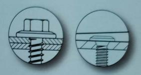
Liplock fixing screw's head height is low, so does not interfere to roof steel after being used.
